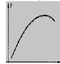
Approximation of a trajectory by linear interpolation
